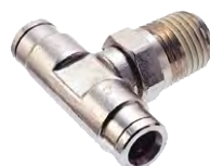
Swivel male centre tee 12467 O/D tube to male NPTF thread
